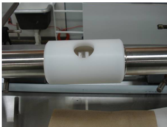
Figure 7. Offline measuring cell for Spectro::lyser™
