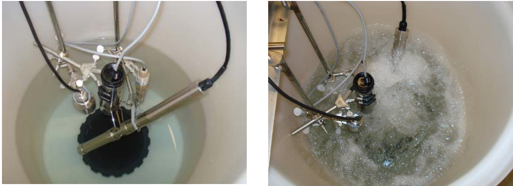
Figure 4. Tank equipped with diaphragm aerator
