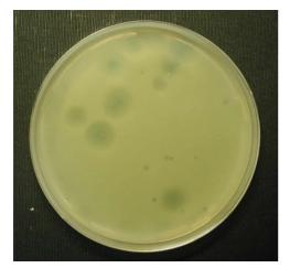
effluent samples with peptone-salt-solution or 1XPBS. Mark petri dishes with sample ID, volume and dilution. Add 1 mL of the wastewater sample dilution (room temperature) to the test-tube. Add 1 mL of Log-phase host bacteria (ice-chilled) and mix gently by avoiding air bubbles. The content should remain molten in the water bath. Do not let the inoculated test tubes longer than 10 min in the water bath. Pour the content onto a labelled MSA agar plate. Do at least 3 duplicates per dilution.
