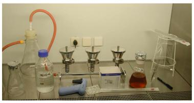
EN ISO standards are adapted to whole effluent of wastewater treatment plants. The detection of *E. coli* and coliforms bacteria are performed according to EN ISO 9308-1:2000, of intestinale enterococci according to EN ISO 7899-2:2000.
