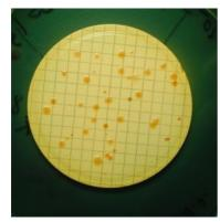
samples with 1x PBS. Mark agar plates with sample ID, volume and dilution. Filter at least 3 subsample volumes of each dilution (25-50mL) through the membrane filter. Place the membrane filter on TCC-agar plate without formation of bubbles between membrane and agar surface. Invert the dish and incubate at  $36 \pm 2 \degree$ C for  $21 \pm 3h$ . If no typical colonies get visible, extent incubation time to  $44 \pm 4h$ .
