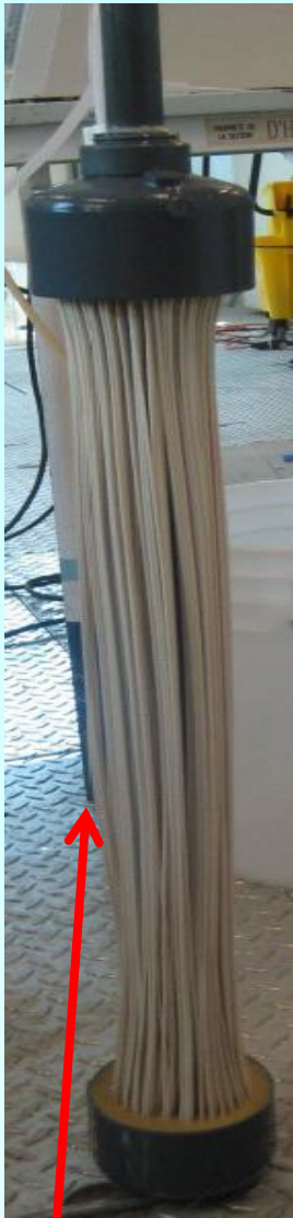
Zenon hollow fibers (ZW-10, 0.04 \mu\text{m} )
